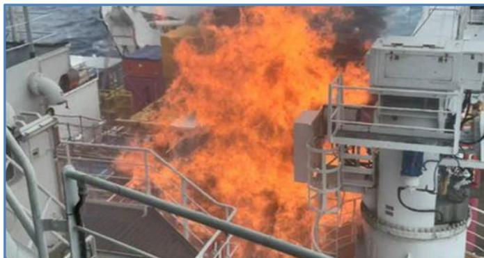
system, crew fatigue, and the design of the ship itself, contributed to fuel oil overflowing into the engine room. The ignition of this overflowing fuel oil, either from contact with a hot surface or an electrostatic discharge resulted in the fire. Among eight safety issues identified, the ATSB found the ship's classification society, Bureau Veritas, had approved the ship's fuel oil settling tank's air vent pipe being positioned within the engine room's exhaust ventilation casing.
