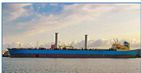
Maersk Tankers is testing the use of wind power to fuel its ships, a new technology it says can cut fuel consumption by up to 10 per cent and help the industry reduce polluting emissions. The move comes as the global shipping industry is suffering from rising oil prices and preparing for fuel costs to rise further by around a quarter, or some \$24 billion, in 2020 when new rules limiting sulphur kick in.
